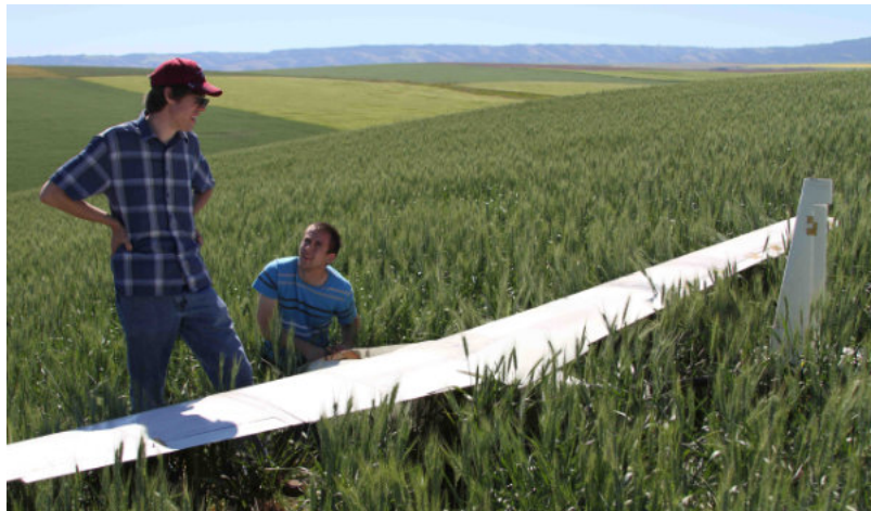
Students with Washington State University's HYPER lab test fly Genii, the first liquid hydrogen fueled drone built by a university team. Photo Courtesy of the Hydrogen Properties for Energy Research (HYPER) Laboratory
